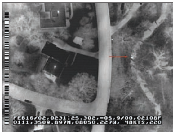
Figure 72: Aerial thermography showing sewage leak
