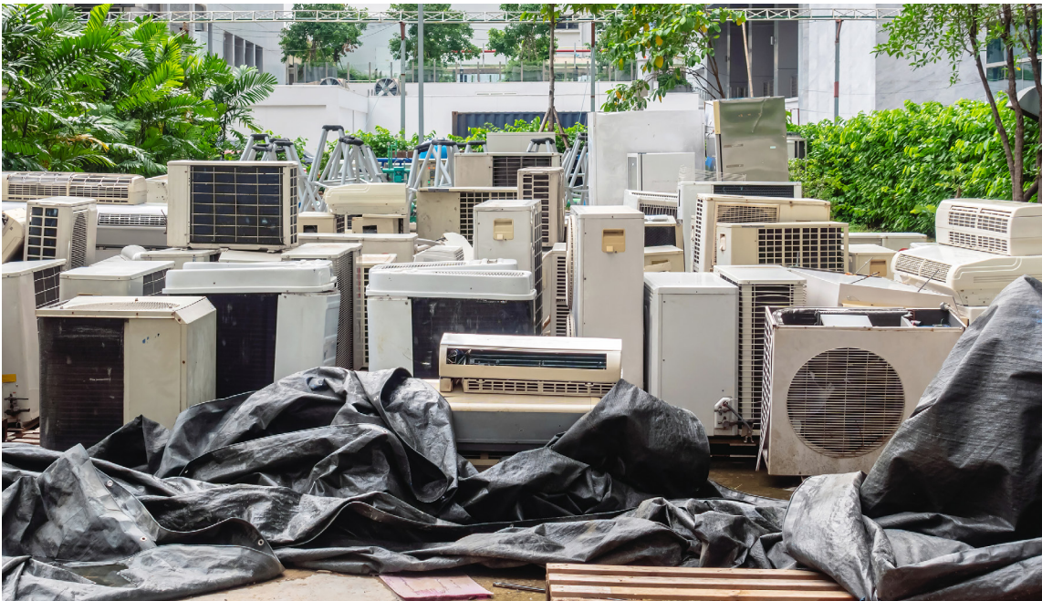
A single air conditioner can hold up to 2 pounds of R410A.
